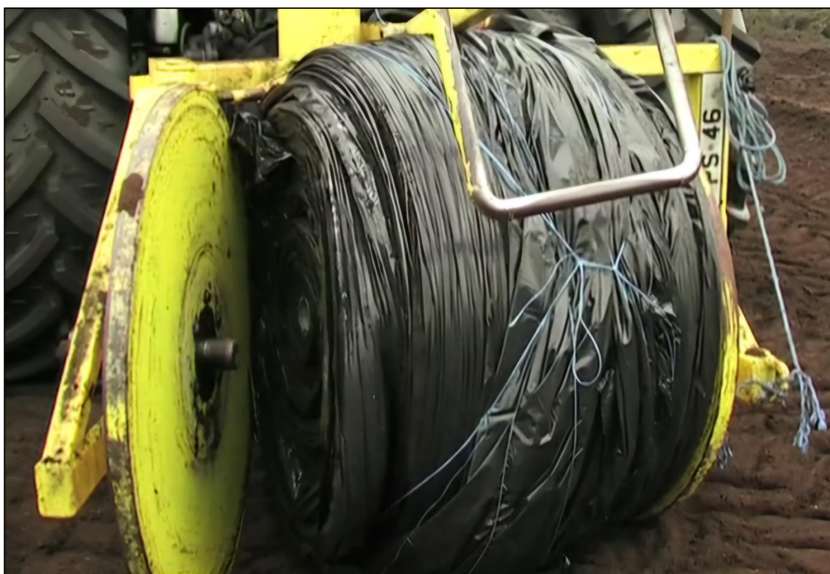
Plate 4- 34 Polywrapper with the frame opened to allow access to the collected bale of polythene
